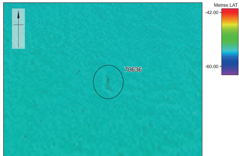
Multibeam echosounder image of dark reflector 70636 , measuring 5.4 x 1.6 x 0.5 m (x1 vertical exaggeration)
